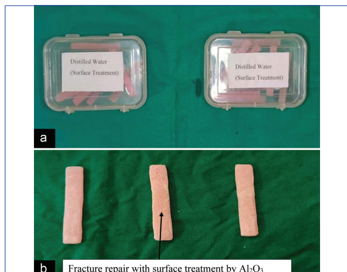
[Table/Fig-5]: Group B: A) Surface treatment with airborne particle abrasion process with 100 μm Al 2 O 3 for 10 second at a pressure of 0.2 MPa from a distance of 10 mm after fracture; B) Fracture repair with surface treatment by Al 2 O 3
